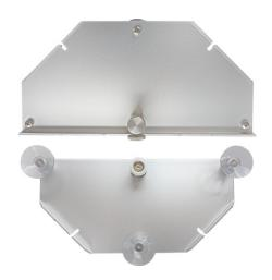
Gluing gauge for gluing the glassbreak sensors. The gauge is designed to ensure the distance from the sensor to the window frame. Furthermore, the gauge ensures constant pressure on the sensors during the curing process of the adhesive.
