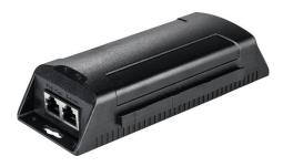
Minimise the need for cables when installing IP cameras. Using the Power over Ethernet (PoE) injector, the data and IP camera power supply are fed into an Ethernet line. Power is then supplied exclusively via the network cable - a separate power line is no longer necessary. Additionally, you are no longer reliant on an available power supply (socket etc.) when selecting the camera location.
