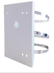
Using the pole mount, selected tube cameras (TVIP91600, TVIP92600, TVIP92610) can be attached in inaccessible places or perfectly positioned on high masts as overview cameras. The cameras are screwed on to the mount with the installation box TVAC31390, with the mount in turn easily installed on masts with a diameter of 130-165 mm.
