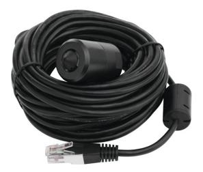
The tube-shaped camera module is a required accessory for the Dual Flex Encoder IPCS10020. The mini module measures just 40 x 26 mm and has an 8 m cable for connection to the encoder, which runs from the back of the device. With an angle of view of 57°, the 3.7 mm pinhole lens gives a focused view of selected areas of a room or into corridors.
