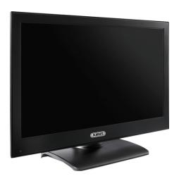
The 23.6" LED monitor displays Full HD 1080p images in 16:10 format. This makes it suitable for displaying megapixel surveillance pictures, as well as use with HD SDI cameras (HDMI converter required). All settings can be conveniently made using the multilingual on-screen display (OSD).
