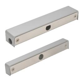
Surface-mounted housing and counterpart for the locking element AZSE10000 and AZSE10100, if it is not possible to mount the locking element in the door frame. The magnet for activating the SpE internal magnetic contact, as well as the additional magnetic contact is included in the counterpart.
