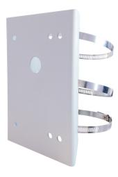
Using the pole mount, selected tube cameras (TVIP91600, TVIP92600, TVIP92610) can be attached in inaccessible places or perfectly positioned on high masts as overview cameras. The cameras are screwed on to the mount with the installation box TVAC31390, with the mount in turn easily installed on masts with a diameter of 130-165 mm.
