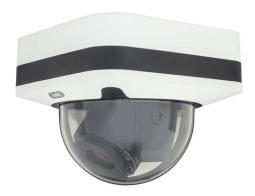
The IP Dome provides video streams in 2 MPx resolution with up to 30 fps. The light-sensitive Sony image sensor proves itself in extreme light situations. The camera provides detailed images in almost total darkness and masters the extreme challenges in a backlight situation due to the outstanding WDR function (~ 150 dB).
